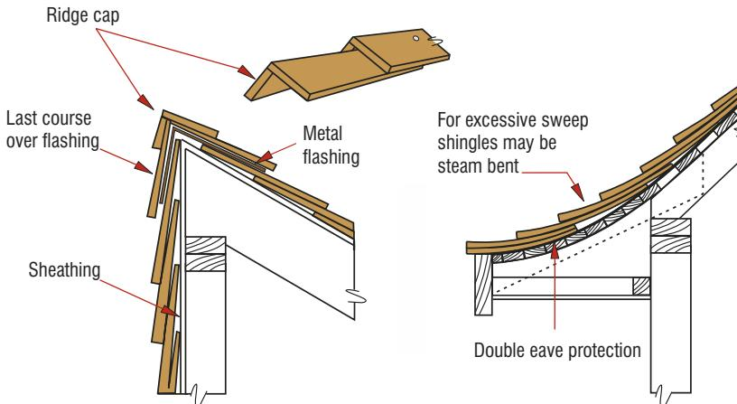
**Figure 11: Apex Roof Juncture**
